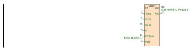
The host PLC reads the 4-channel temperature values of H04RC by Modbus read instruction MODR, the start address is 10H (hexadecimal), that is, the decimal value is 16. When the communication is successful, M0 is ON, the temperature values which are read back will be stored in V0-3, V0=235, indicating that the actual temperature of the first channel is  $23.5^{\circ}$ C, the same as V3=867, indicating that the actual temperature of the fourth channel is  $86.7^{\circ}$ C.
