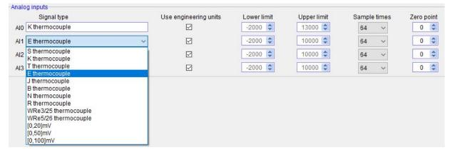
In this way, after configuration, as long as connect the K-type thermocouple to channel 1, then directly read AI0 register value, AI0
